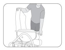
Loosen the knob on each leg (about 1 1/2 turn), pull the knob and slide the leg into the tube in order to obtain the desired height. Align the holes and release the knob. Tighten the knob properly.
