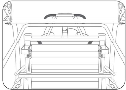
2. Using a  $\frac{1}{2}$ " [13 mm] wrench, loosen the 4 bolts under the seat structure that go through slots that control the seat's depth. **WARNING: DO NOT REMOVE THEM ALL THE WAY.**
