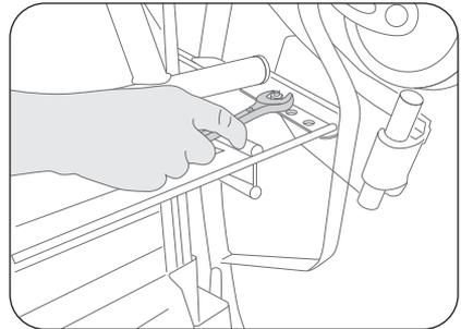
3. Position the seat bracket at the desired height. **MAKE SURE BOTH SIDES ARE AT THE SAME LEVEL.** Put back the 4 bolts without forgetting the flat washers and the lock washers. Tighten properly.
