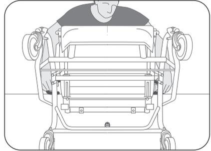
2. Using a  $\frac{1}{2}$ " [13 mm] wrench, remove the 4 bolts (2 per side) that hold the seat support.
