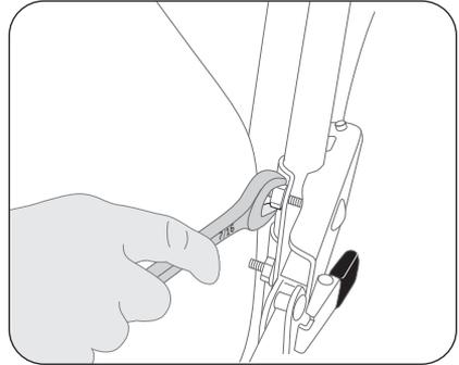
3. Position the lateral supports at the desired height. Retighten the nuts.
