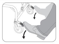
WARNING: BEFORE HANDLING AN OCCUPANT OR MAKING AN ADJUSTMENT, BOTH BRAKES MUST BE APPLIED AS SOON AS THE CHAIR IS NOT USED FOR MOVING TO ENSURE STABILITY
