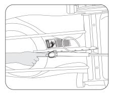
4. Reposition the gas spring in the correct place. Then, reinsert the locking pin and secure it with the wire retainer snap.
