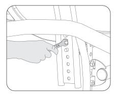
2. Position the armrest at the desired height and replace the bolt, without forgetting the flat washer and the lock washer.
